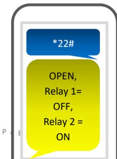
Send the SMS as shown, and the unit will reply showing the status of the input limit switch (if used), and the relay..
